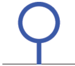
POST AND LOOP One rack element supports two bikes.
