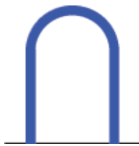
INVERTED "U" One rack element supports two bikes.
