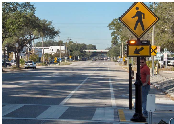
Example of a rectangular rapid flashing beacon (RRFB), used for crossing improvements at uncontrolled approaches.
